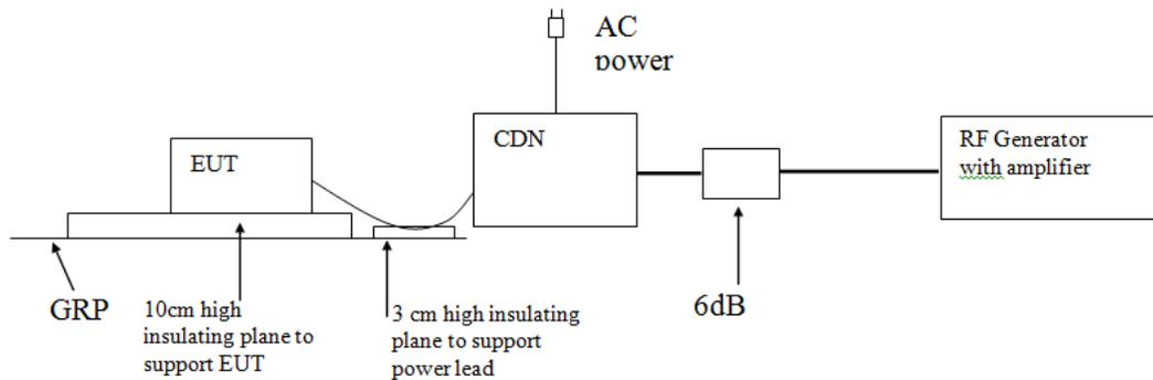
**8.2.2 Test Setup and Procedure**
