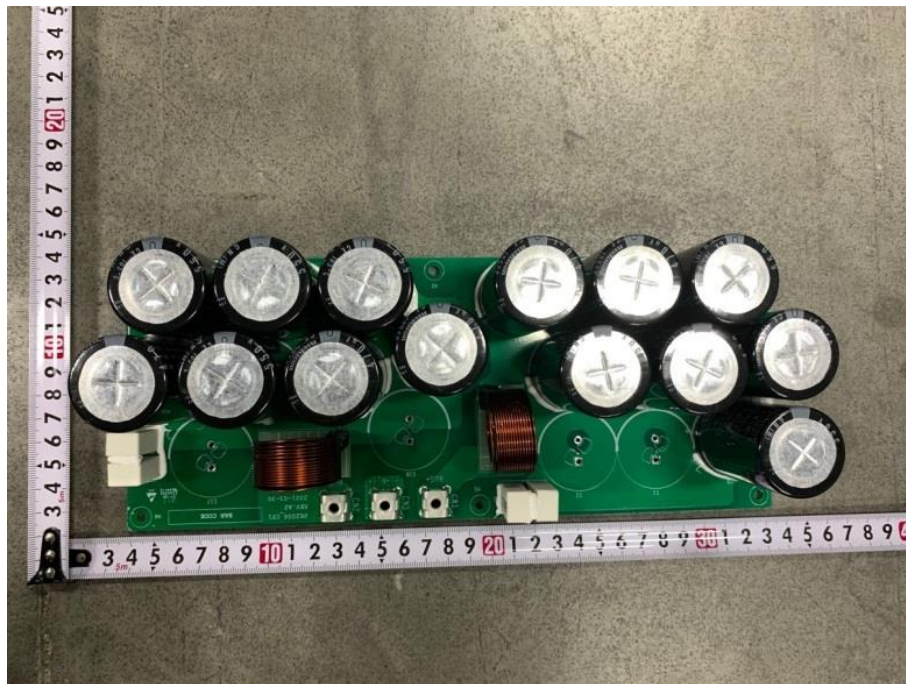
Capacitor board(Components side)
