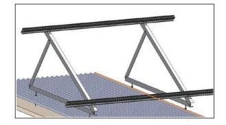
Installation of the splice to connect multiple rails together. Slide the splices on the rear side of the pre-assembled rails halfway to the side. Fasten the first M8 bolt firmly using the Allen key. Now slide the next rail segment into the splice. Tighten the second M8 bolt .The connection is finished.
